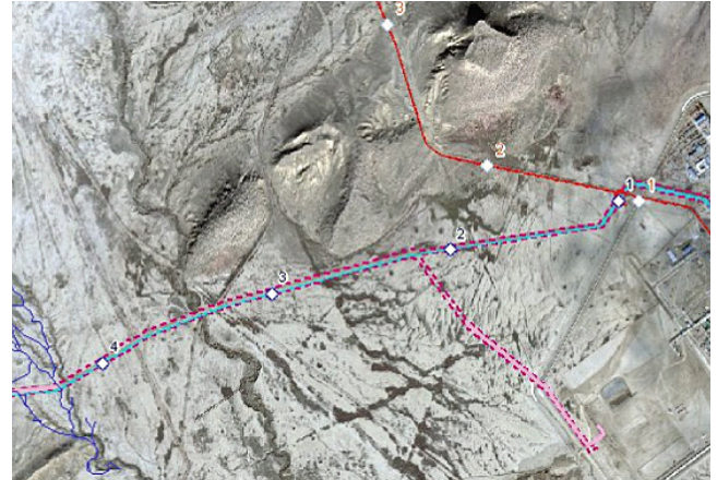
BP Azerbaijan operates four pipelines that transport crude oil from the Caspian Sea to the Mediterranean and Black seas. Pipeline engineers use satellite imagery to help monitor changes to the landscape over time.
